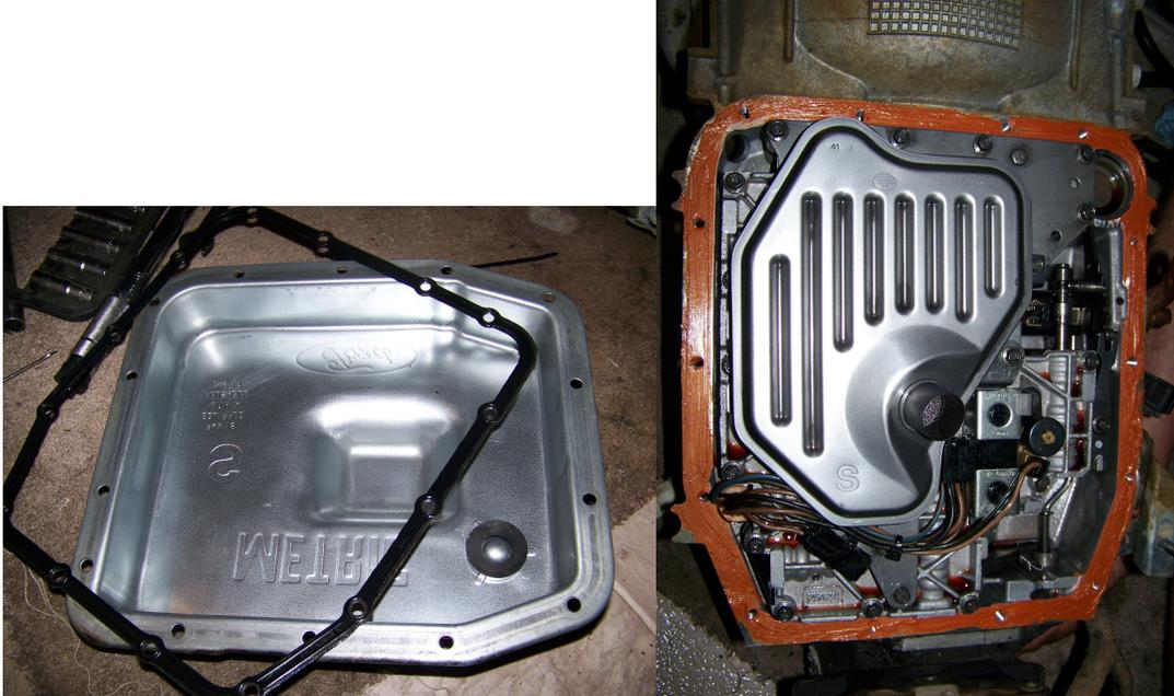
7. Torque your pan bolts flip the transmission over. Install the MLPS and the 94 Exterior Harness. Make sure you line up the MLPS properly. Switch out the Speed Sensor. PUT IT BACK IN YOUR CAR.
