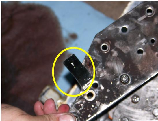
**\* Note there is a grounding clip on the 994 TCC solenoid bolt. You will need it. The 98 does not have one. Remove what I believe to be the Trans Temp sensor. Just gently pry it off the plate. If you break the clip don't freak out. It's no big deal. I broke the clip to.**
