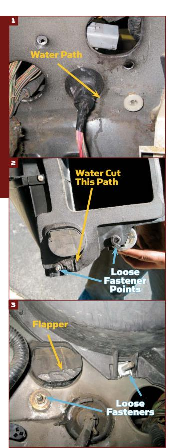
the recirc duct (which is bolted to the inside of the bulkhead right next to the A/C plenum), then back out a special spout with a top-hinged rubber flapper that allows the water to find its way to the ground. The spout and flapper aren't easily visible without the fender splash shield removed, but you can raise the vehicle, bend the bottom of the fender splash shield slightly forward and see this water exit point with a flashlight if you want to.
