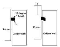
The conventional caliper produces a given amount of distortion which pulls the caliper piston back into the caliper bore only slightly
