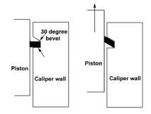
The low drag caliper flexes twice as much and pulls the caliper piston back into the bore twice as much.
